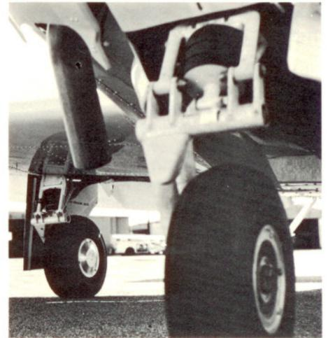
Rugged Mooney gear has no fancy hydraulics or oleos to run up shop bills. Positive-action energy-absorbing electric gear retracts or extends in just seconds.
